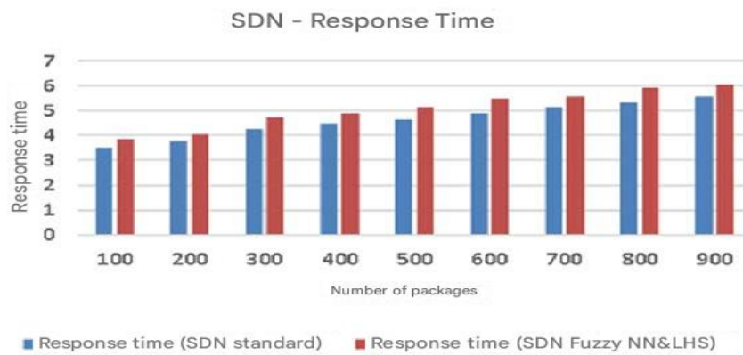
Fig. 5. Comparison of the response time of a network with a traditional SDN architecture and a network with an analysis and clustering subsystem
