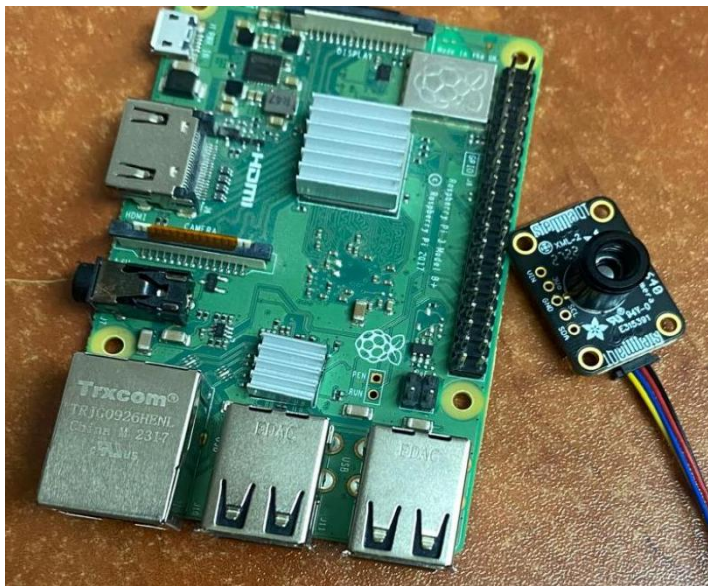
Fig. 3. Raspberry Pi processing unit used for sensor data processing.
